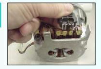
To install (PTC) motor starters, push female terminals over pump motor terminals 2 & 4. terminals are different sizes to match the smaller motor terminal 4.
