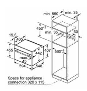
If the compact appliance is installed beneath a cooktop, the following countertop thickness (possibly incl. substructure) must be observed.
