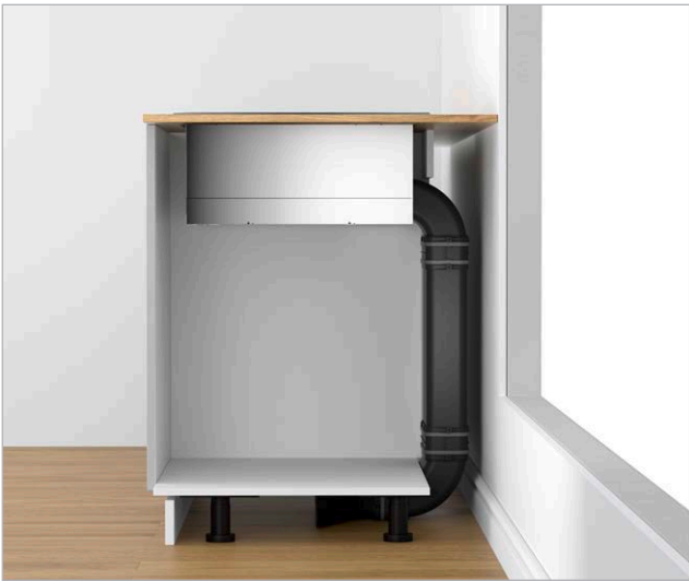
Next to uninsulated exterior walls ( \mu \geq 0,5 \text{ W/m}^2 \text{ }^\circ\text{C} ), a partly or fully ducted recirculation configuration is recommended in order to minimize any potential condensation risk.
