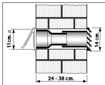
The appliance can be installed on a permanent basis using window/wall Optional Accessory, reference B1 RKZ 06009, available from your supplier.
