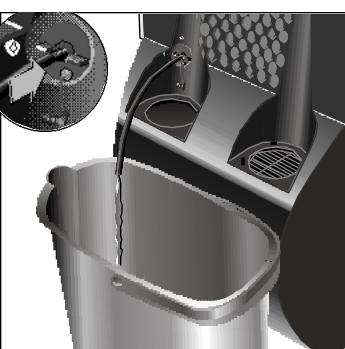
**Do not forget to put the plug back in place on the drainage stopcock and to turn the stopcock 90° in a clockwise direction before setting the appliance to the temperature control setting. The appliance will shed water if you fail to do so.**
