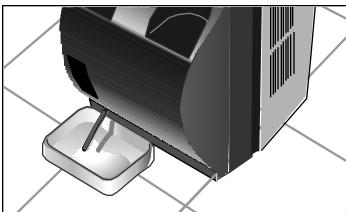
There are castors fitted on your appliance to make moving it easier. If it is necessary to tilt your appliance in order to move it, then the internal water tank must be drained first. To do this, connect drainage pipe to stopcock at the bottom of the appliance.
